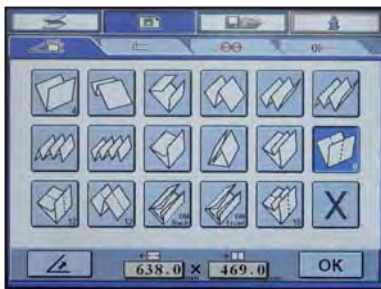
Setup is completed by selecting the desired fold pattern and inputting the sheet size.
