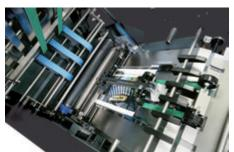
Folding roller and press roller gaps are automatically adjusted according to the booklet thickness. The jog sensor detects jog faults and rejects any errored booklets to the reject tray. Sheets are firmly registered with tail edge and top-bottom guides to provide accurate folds.
