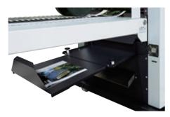
Errored sets are rejected to the reject tray so that only correct booklets are delivered to the conveyor.
