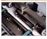
Scoring positions are automatically set to the input thickness. Scoring depth is easily adjusted to accommodate a wide range of cover stocks and thickness. This insures a professional bind quality with sharp, square spine corners.
