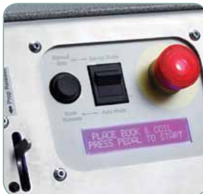
LCD Screen communicates machine status at all times.
