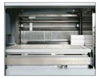
Maximum stack height is 254 mm (10"). Stacked sheets are delivered to the output conveyor for easier handling or downstream finishing.
