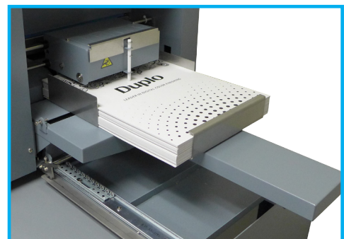
Automatic sheet feeding system
