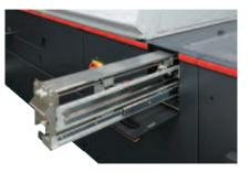
Optional cover slitting device to slit both edges of the cover to eliminate cover over hang for easy handling and increased accuracy at the three knife trimmer.
