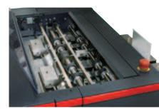
Optional cover reject device is available to reject the cover in case the cover does not match the book block.
