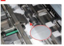
The scoring width and position are automatically set-up according to book block thickness and cover registration. Scoring is performed on thick covers for professional binding with sharp, square spines and hinge scores.
