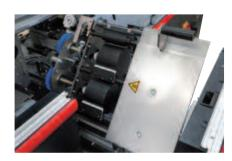
The application drums and back spinner lift and latch to provide easy access for cleaning of the tank.
