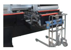
Sliding rail glue tank for easy replacement. Pull out the tank and remove it with the optional lifting trolley.
