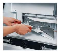
SAFE BLADE CHANGES Blade changes can be made without removing machine covers. Handy blade changing device covers the cutting edge of blade.
