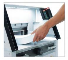
IR SAFETY CURTAIN IR light beam safety curtain covers work area to ensure the highest level of operator safety.
