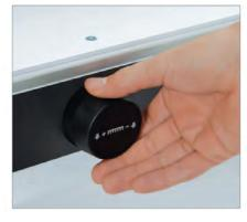
**ELECTRONIC HAND WHEEL** The electronic hand wheel, with infinitely variable speed control, is used for manual back gauge positioning.
