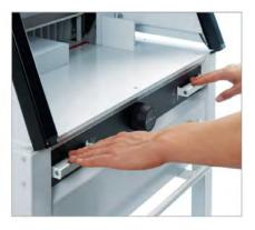
EASY CUT BLADE ACTIVATION BARS Patented EASY CUT blade activation bars ensure true, two-handed operation and allow blade and clamp to be activated independently.
