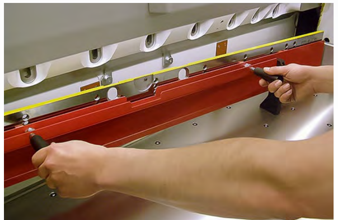
Blade changes are safe, quick and easy. This image shows the blade mounted in the protective guard after it was lowered by the knife hoist.
