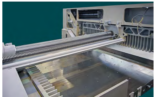
The backgauge is rigidly-mounted from above so there is no need for a slot in the table which permits smooth sliding of stacks. No table slot belt to get caught on like on other brands.
