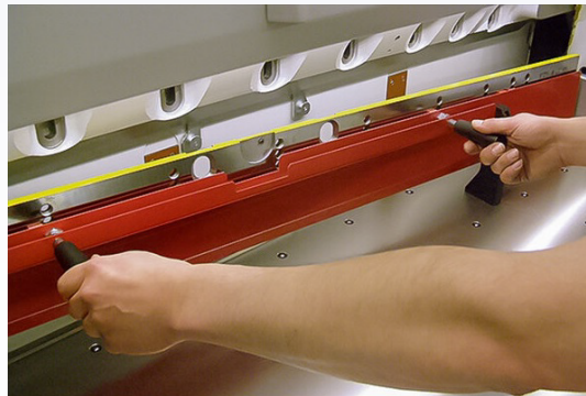
Blade changes are safe, quick and easy. This image shows the blade mounted in the protective guard after it was lowered by the knife hoist.
