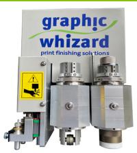
Dual RCT : Rotary Cutting Tools cuts up to 1.8mm
